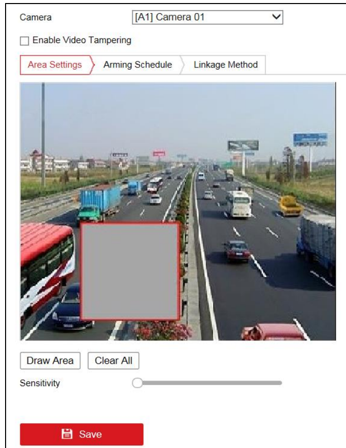
Figure 7. 11 Video Tempering Alarm Settings
